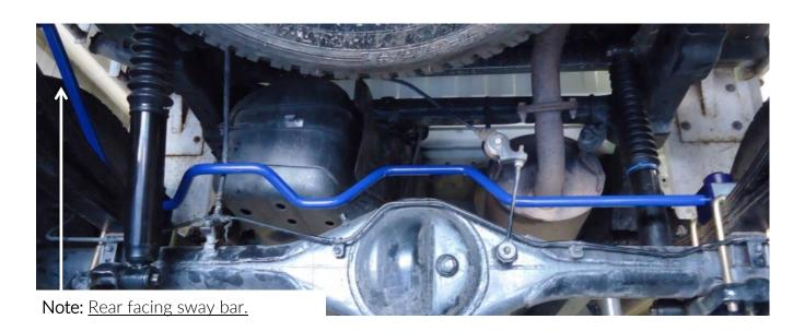
Recheck positioning and Torque all bolts.
