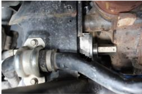
Figure 3 – Use threaded rod to pull the bush into place
