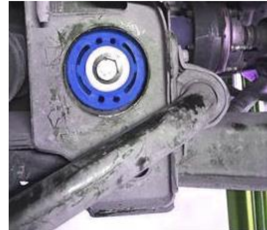
Figure 5 – Rear position view from wheel well SPF5215 bush in housing – note voiding orientation
