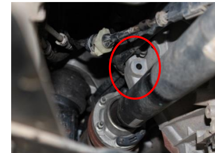
Figure 2 - Location of gear selector and its attaching point to transmission
