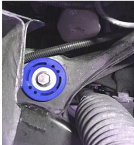
Figure 4 – Front position view from wheel well SPF5215 bush in housing – note voiding orientation
