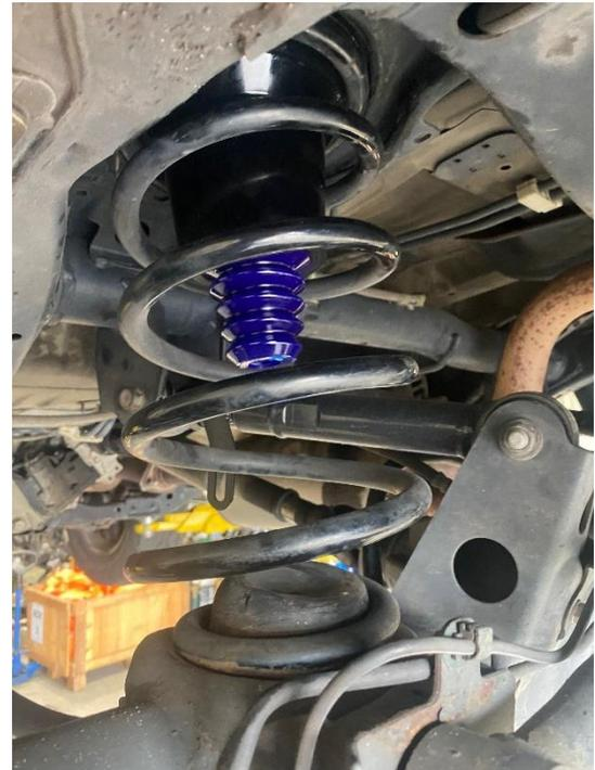
Figure 01 – Completed Installation of Bump Stop
