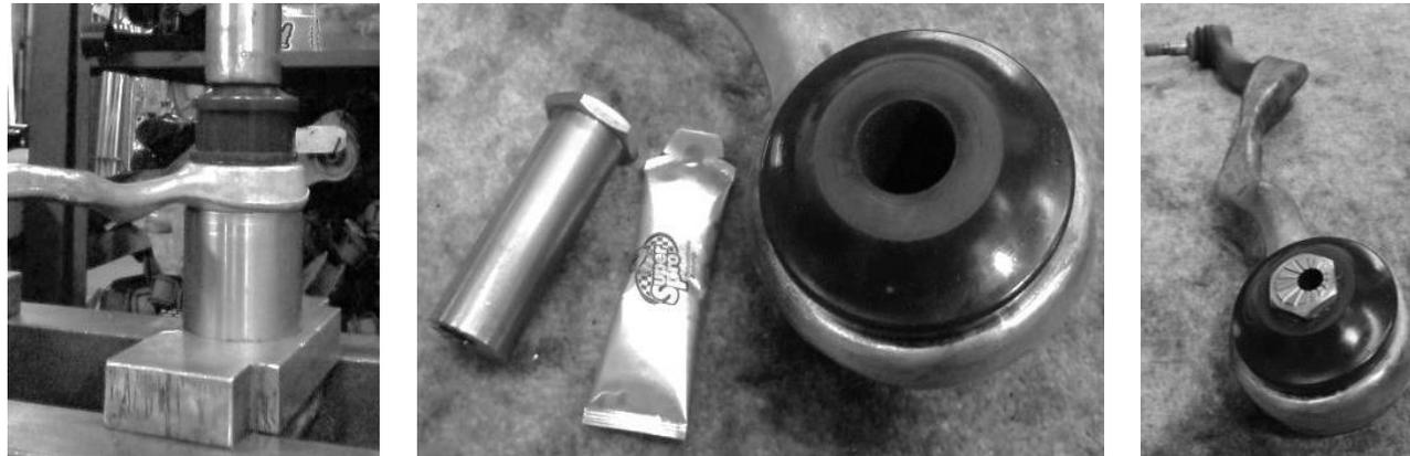
Figure 1: SuperPro Polyurethane Bushes and Crush Tube Assembly in Arm
