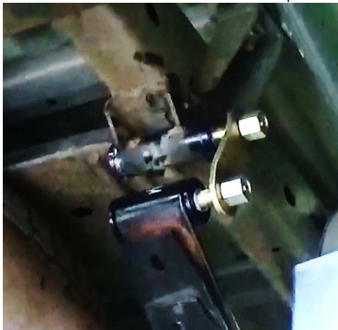
Figure 5: Installing greasable shackle
