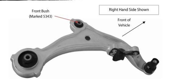
*Note:* Polyurethane bushes must be fitted to both sides of the vehicle.
