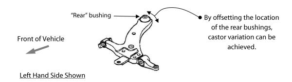
*Note:* Polyurethane bushes must be fitted to both sides of the vehicle.
