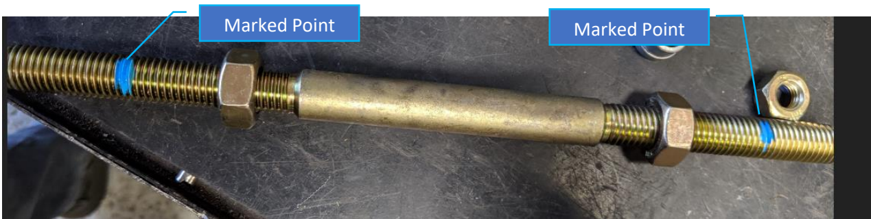
Figure 2. Link Rod displaying Marked Points
