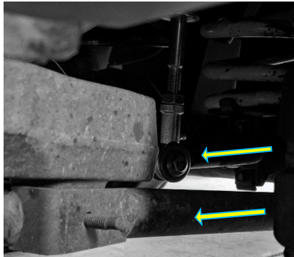
Figure 6. Parallel Link Pin and Trailing Arm.
