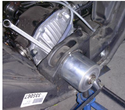
Figure 2 – Insertion of new bush
