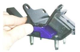
3. New insert bushing must be installed centralized to the mount.
