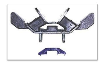
2. Use slight amount of force to push the insert bushing into the void, as per photo No2.
