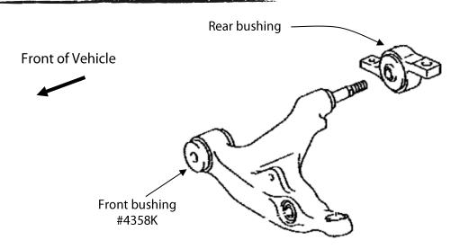
**Note:** Polyurethane bushes must be fitted to both sides of the vehicle.
