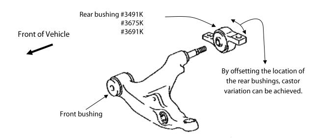
**Note:** Polyurethane bushes must be fitted to both sides of the vehicle.
