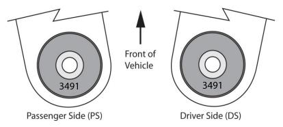
**Kit #3675K** – to counteract a slight pull to the left (approx. 0.8 deg. change) Single Offset – (passenger side castor increase & drivers side no castor change)
