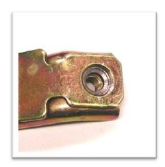
• With the riveted area removed, the two halves of the bracket can be gently pried apart, enabling the original rubber bushes to be removed;
