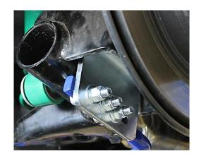
Fit the Sway bar to the brackets using 3 cap screws per side. Note the 2 mounting positions below;
