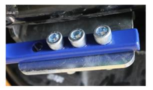
Tighten all bracket bolts first and then tighten the bar bolts. Torque all nuts and cap screws approximately 46Nm;
