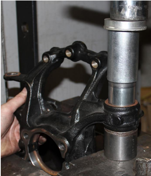
Figure 3: O.E Bush Removal from the rear hub
