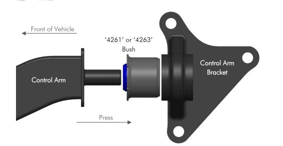
*Note:* Polyurethane bushings must be fitted to both sides of the vehicle.
