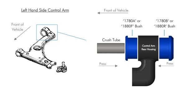
Note: Polyurethane bushings must be fitted to both sides of the vehicle.
