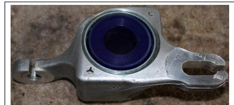
Make sure that the rear bush sits flush on the bracket side with wording
