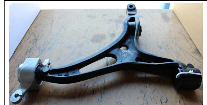
Left Hand Arm Shown-Complete with SuperPro Bushes Installed
