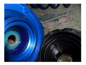
Using the included grease packet, liberally grease the exposed blue polyurethane isolator on the underside of the TRC5000 mount;
