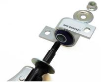
Insert the smaller diameter washer ensuring that the inner race section of the washer faces the bush.
