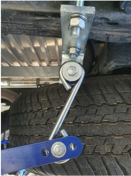
Figure 3: Sway bar Installation (Left Hand Side Shown)
