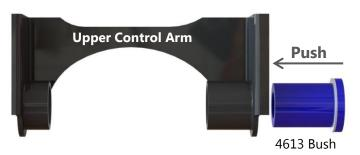
2. Press the supplied crush tubes onto the cross pin first, and then, install the cross pin into the control arm.
