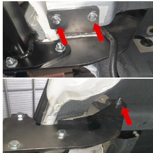
**\* Note: 3-piece bar pictured. 1-piece bar endplates fasten to the chassis. Please disregard the 3xbolts pictured attaching the main bar.**
