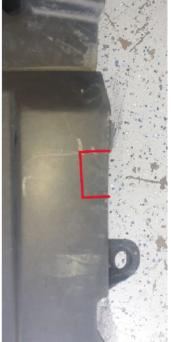
c. Cut the bumper using an air saw or similar cutting device ensuring to deburr the cut edges.
