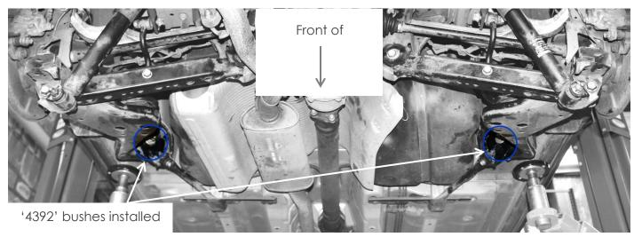
Note: Polyurethane bushings must be fitted to both sides of the vehicle.
