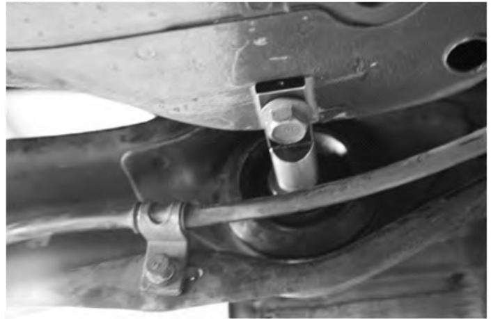
10. Tighten all bolts to OE specification, and bleed brakes if required.
