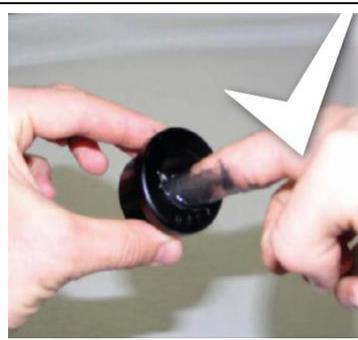
Lubricate internal bore.
