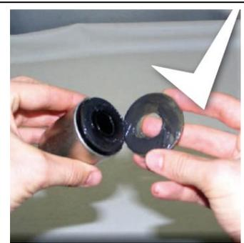
Lubricate shackle plate/working surface (hardware if supplied).
