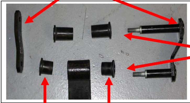
A center sleeve may or may not be required at this point in the bushing kit as some bushings may run directly on the shackle pin or spring eye pin.
