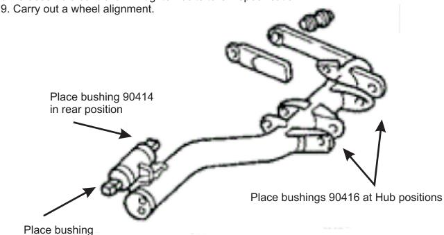
N.B: It is recommended that a licenced workshop or tradesperson carry out the above procedure and that workshop manual and relevant safety procedures are followed in addition to the above.
