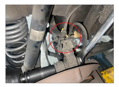
• Access the inner mount bolt with a ratchet and socket. Loosen nut from rear side.
