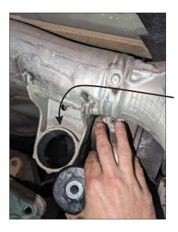
Remove the original bushings including the outer shell. This can be achieved with a threaded puller with appropriate size steel cups.
