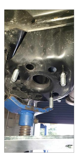
Use a small drill bit for a pilot hole. Then finish off with a M10 drill bit.
