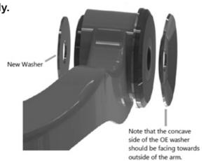
Tip - the bushing supplied being free spinning offer the ability to tighten the long bolt while the wheels are hanging.
