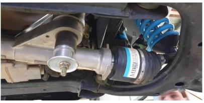
Once the OE bushing is removed, clear up the bore of the housing to remove any burrs or debris.
