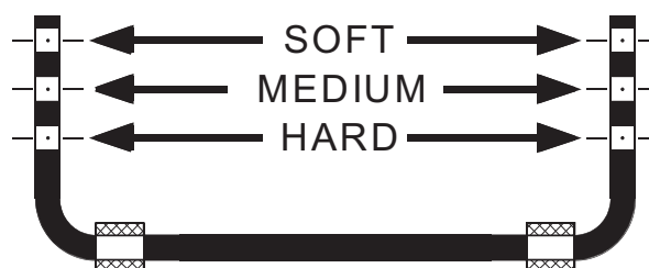
WHITELINE Blade adjustable swaybar - rate adjustment guide
