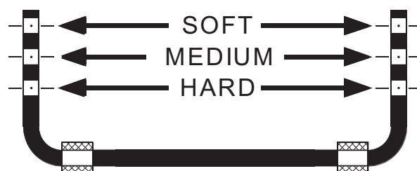
WHITELINE Blade adjustable swaybar - rate adjustment guide
