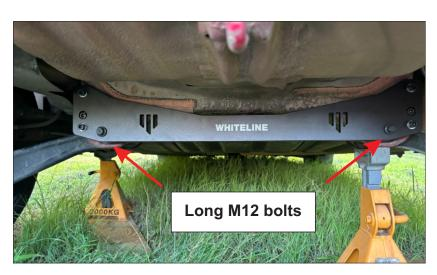
Tighten the M12 bolt to 95Nm/70ft-lbs
