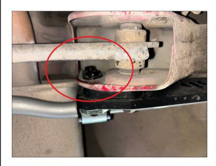
Next - locate the 2x small threaded backing plates. LH image. Using the 2x small M10 bolts, loosely bolt up the backing plates via the 2x recessed holes in the brace.
