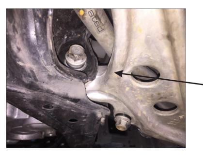
• Loosen inner bushing bolt this will help with lowering control arm down - to remove ball joint.
