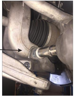
• Loosen and remove Ball Joint bolts from Hub.
