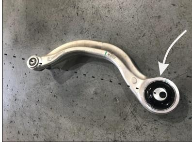
Note - place offset as per LH image - the bushing bolt hole should sit inline with ball joint centre line. (away from ball joint).
