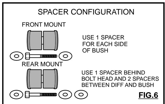
4. Once the OE bushings are removed, wipe eyelets and remove any sharp edges. 5. Insert the supplied 2-piece bushings from either side of each eyelet. Note: Bush voiding to be timed as per figure 4 and 5. Note spacer configuration as per figure 6.
