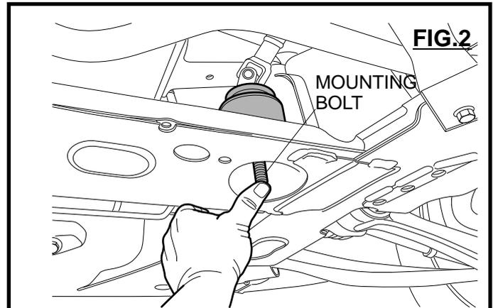
1. Once the vehicle is evenly raised and safely supported, remove the passenger side wheel. Then un-bolt the brake caliper and rotor. 2. Remove the 3 differential mounting bolts and gently push the housing away from the passenger side bushings.
