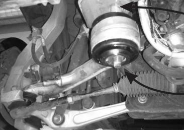
Place washer 52x20x3 on top side of bushing
