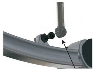
Head light sensor rod - M3 models
