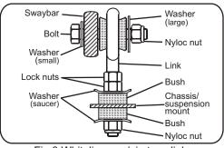
Fig.3 Whiteline eye/pin type link.
