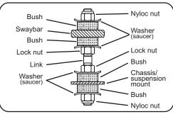
Fig.1. Whiteline double pin type link.
