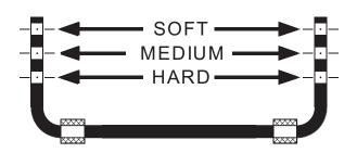
WHITELINE Blade adjustable swaybar - rate adjustment guide
