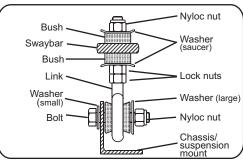
Fig.2. Whiteline pin/eye type link.
