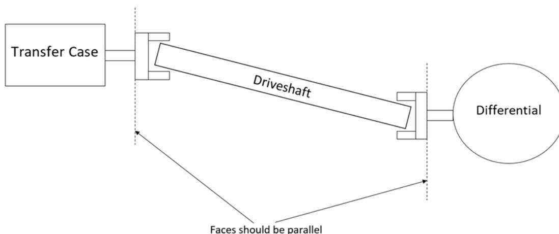
To correct pinion angle, use an inclinometer to measure the difference in angle between the faces on the transfer case and the differential and adjust the trailing arms as required until difference in angle is 0 degrees.
