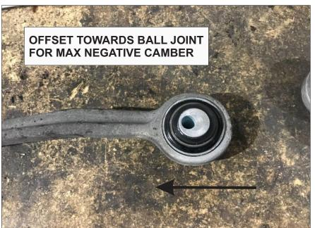
Refer LH image with off-set inner steel tube installed.
