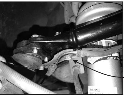
Using original bolts, bolt up ABS wire bracket under arm
