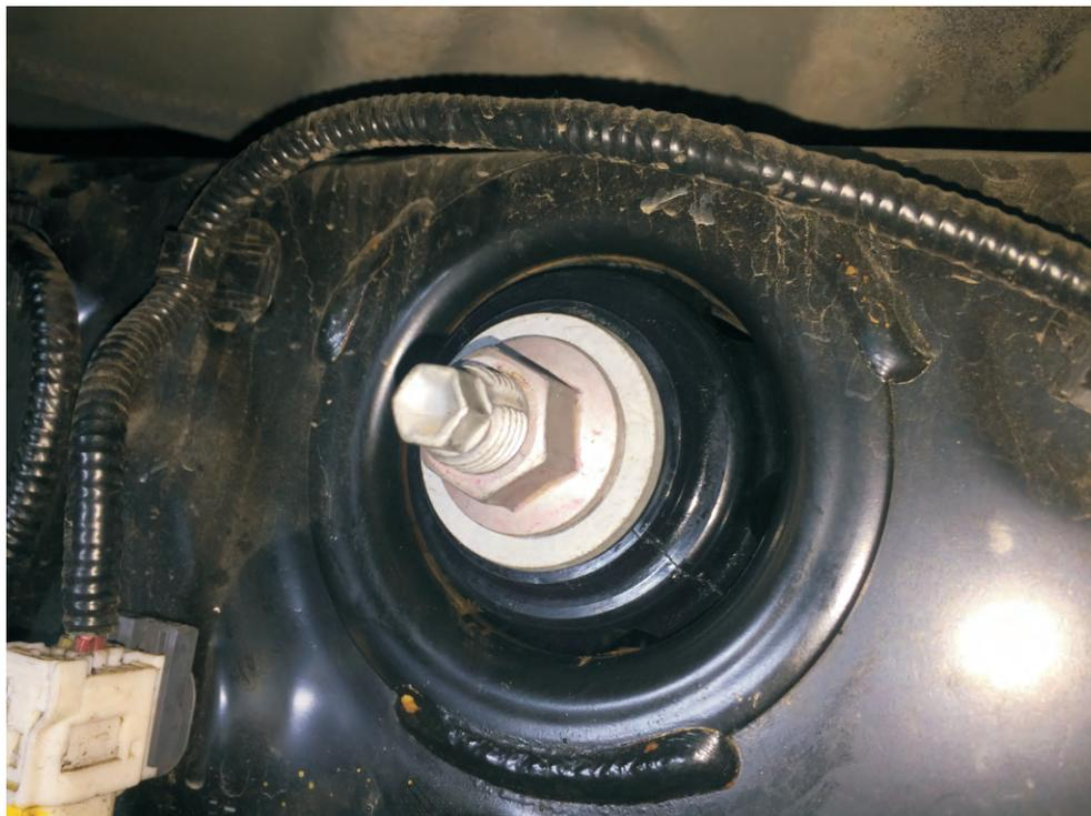
7. Re-use original washer and flange nut - tighten to 80 Nm.
