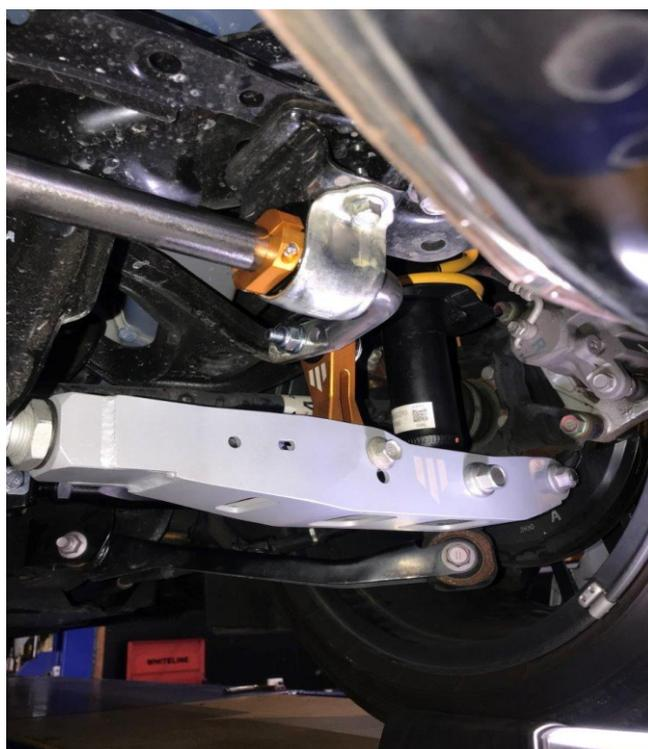
**\*\*IMPORTANT - a wheel alignment will be required immediately after install\*\***
