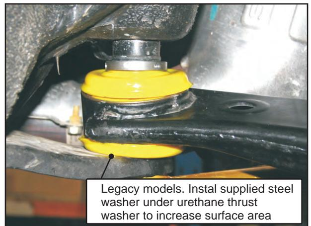
Fig 3 - right-hand control arm, outside view.
