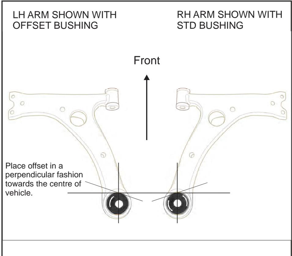
Press bushing in with voiding orientation as per above.
