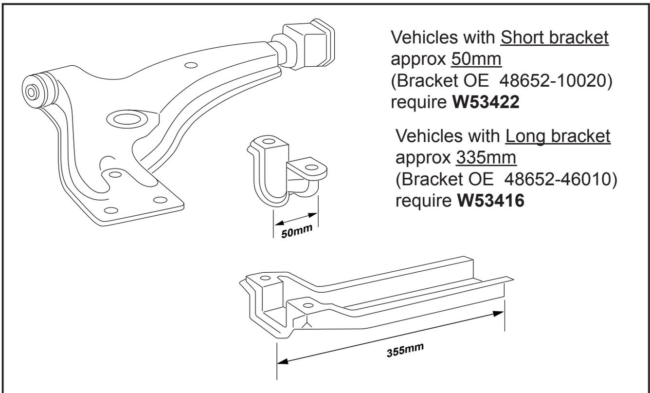
**Special Note** - This Vehicle series can have different rear mounting brackets. Please insure that you have the correct kit for your vehicle. The diagram below shows the different rear mounting brackets and the correct kit part numbers.
